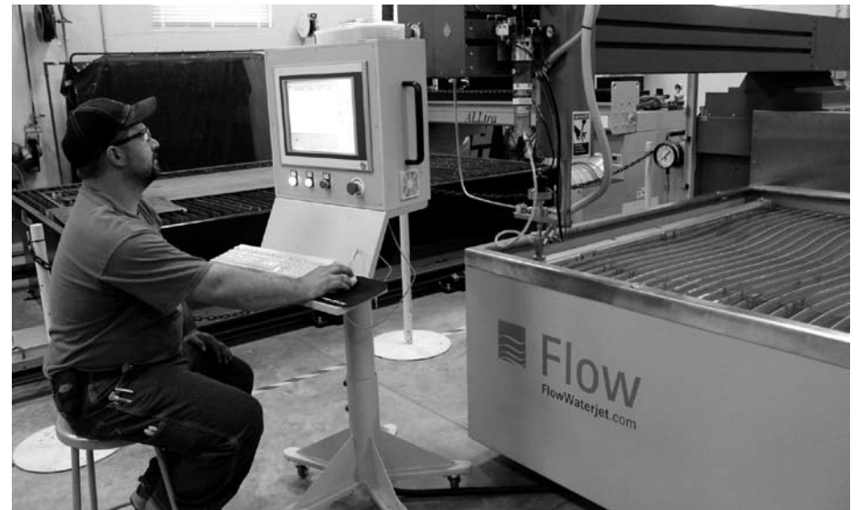
Instructor Assistant Corey Wegner programs the new water jet cutter at the Chippewa Valley Technical College welding show. The equipment uses water under high pressure to cut metal and other materials.
